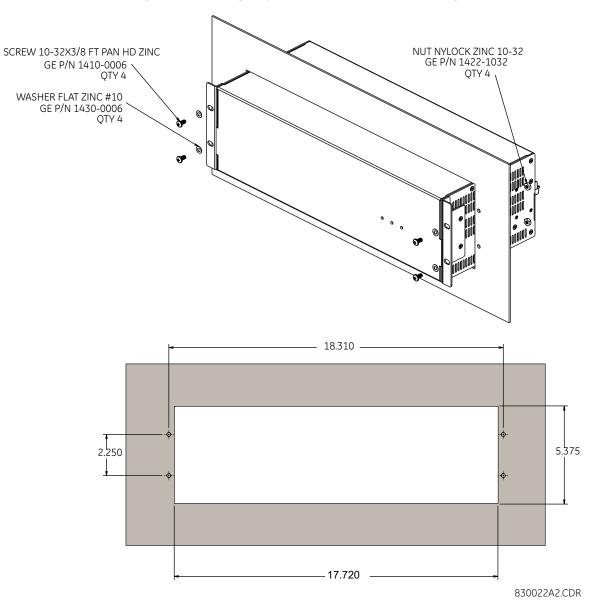
Figure 24: Mounting for panel-mounted GPM-S-G (second generation) (inches)
