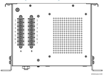
Figure 29: GPM-S-B showing terminal blocks
