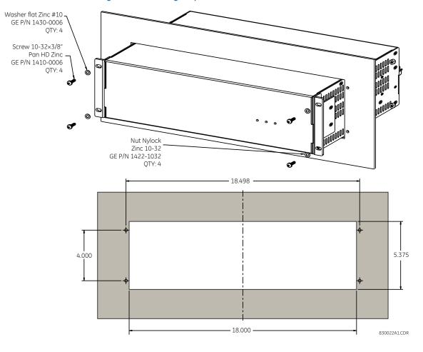
Figure 25: Mounting for panel-mounted GPM-S-G (discontinued) (inches)
