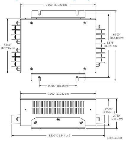
Figure 12: Dimensions for GPM-F-R high-voltage resistor box
