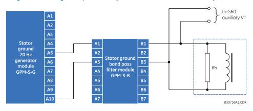
The following figure illustrates how to connect the stator ground 20 Hz generator module with the band pass filter module where the NGT secondary voltage is greater than 240 V.
