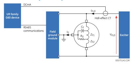
Figure 34: Field ground fault detection
