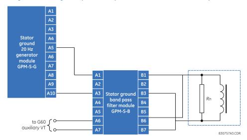
Figure 31: Stator ground protection system connections (NGT secondary > 240 V)
