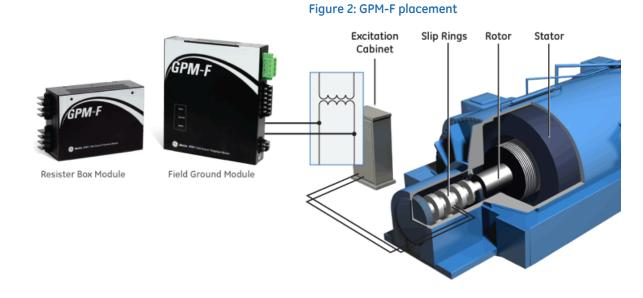
The following figures show placement of GPM-F and GPM-S units.
