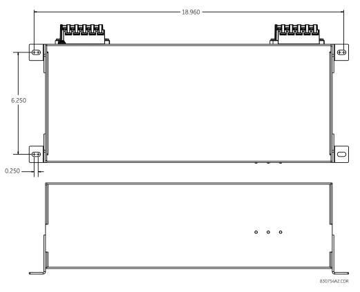
Figure 22: Dimensions for GPM-S-B band pass filter (inches)
