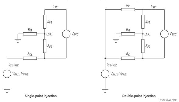
Referring to the single-point injection circuit, the magnitude of  $I_{FLD}$  makes it evident that  $V_{INJ}$  cannot have a significant impact on the voltage drop across  $Z_{F2}$ . Therefore if two values ( $V_{INJ1}$  and  $V_{INJ2}$ ) are injected, the following equations can be written:
