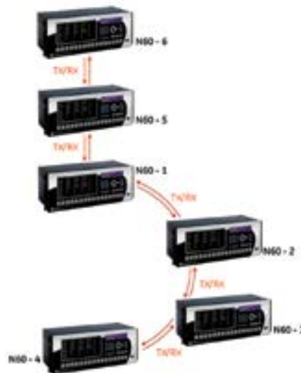
N60's can be directly connected to other N60's in a ring configuration, providing network redundancy as seen in Figure 1, or an open ring configuration to span long distances, as seen in Figure 2.
