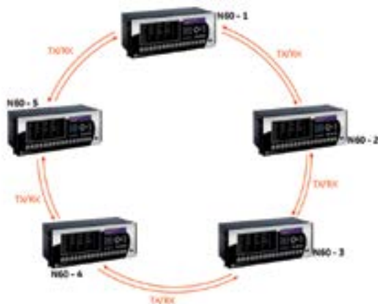
N60's can be directly connected to other N60's in a ring configuration, providing network redundancy as seen in Figure 1, or an open ring configuration to span long distances, as seen in Figure 2.
