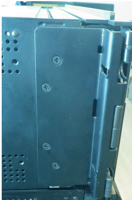
Figure 8-17: Unscrew enhanced front panel mounting bracket on left side
