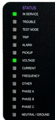
Figure 4-51: Example of LEDs on graphical front panel
