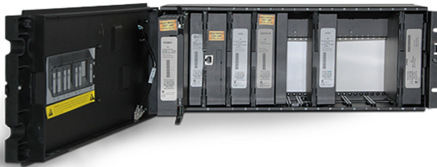
Figure 8-25: Modules inside relay with front cover open (enhanced front panel)
