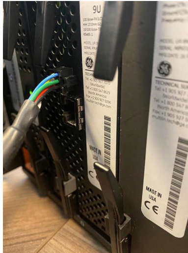
Figure 8-23: Connect graphical front panel to top connection on CPU module
