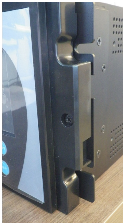
Figure 8-24: Screw to attach graphical front panel to mounting bracket
