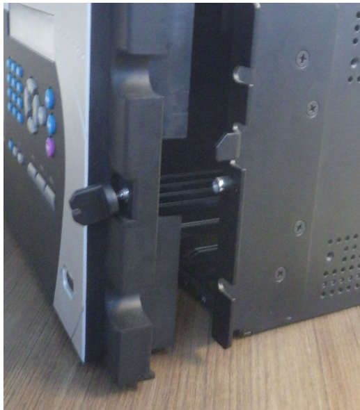
Figure 8-15: Remove enhanced front panel mounting bracket on right side
