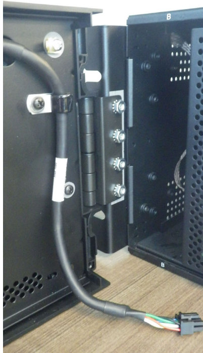
Figure 8-20: Attach to left mounting bracket inside relay
