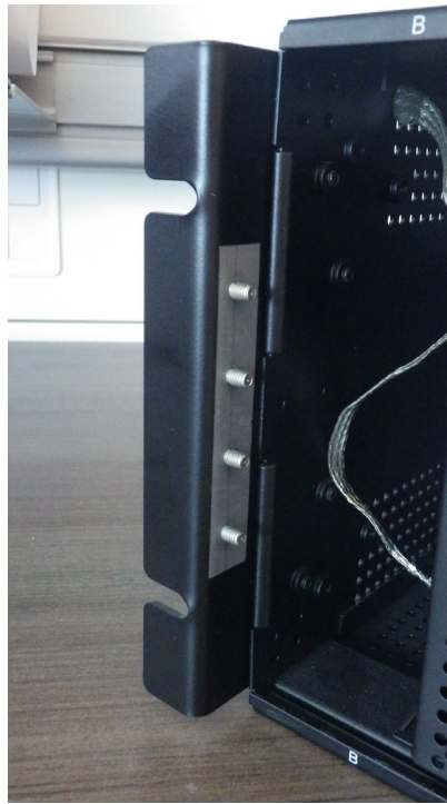
Figure 8-18: Attach mounting bracket on left side (no power supply module in first slot)
