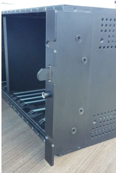
Figure 8-19: Attach mounting bracket to relay on right side
