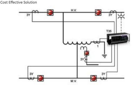
Auto-transformer with breaker-and-a-half on both sides and loaded tertiary.
