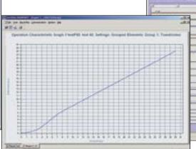
Visualization of differential characteristics allows for setting verification and operation troubleshooting. Analyze transformer faults using both analog and digital power system quantities that are measured and recorded up to a rate of 64 samples per cycle.
