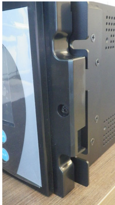
Figure 9-25: Screw to attach graphical front panel to mounting bracket
