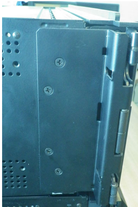
Figure 9-18: Unscrew basic front panel mounting bracket on left side
