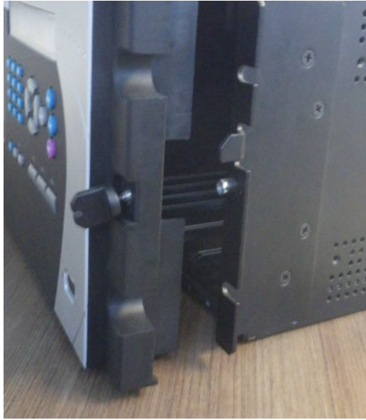
Figure 9-15: Remove basic front panel mounting bracket on right side
