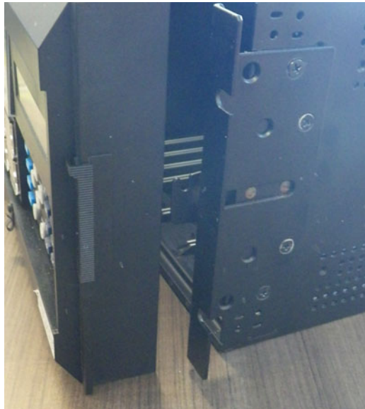
Figure 9-15: Remove basic front panel mounting bracket on right side
