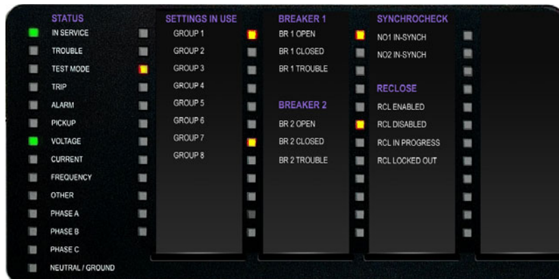
Figure 4-46: Typical LED panel for enhanced front pane
