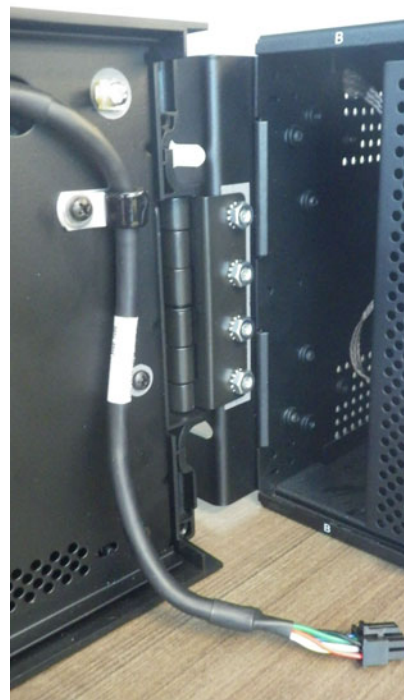
Figure 10-21: Attach to left mounting bracket inside relay
