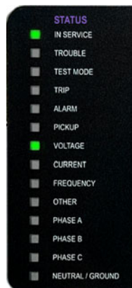
Figure 4-51: Example of LEDs on graphical front panel
